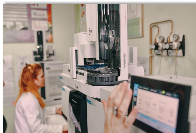
picture 11. Pesticide residues determination (GC-MS/MS)
