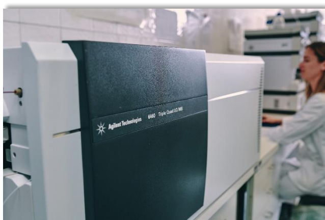
picture 10. Pesticide residues determination (Triple Quad LC-MS/MS)
