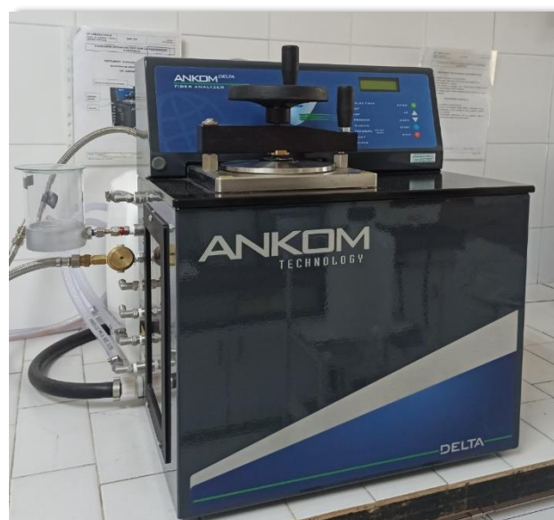
picture 1. ANKOM Delta instrument for the determination of crude fibre - cellulose
