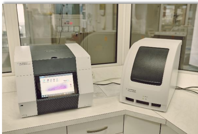
picture 13. Real-time PCR for GMO determination
