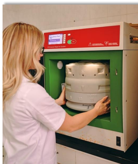
picture 12. Sample preparation by microwave digestion for the determination of metals and metalloids using ICP/MS
